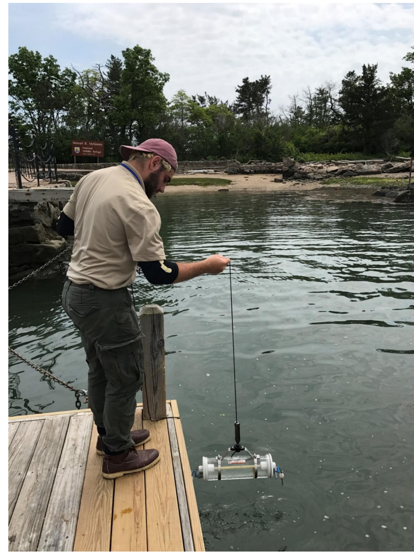
Ian Bergemann using a Beta Horizontal water bottle for sample collection
