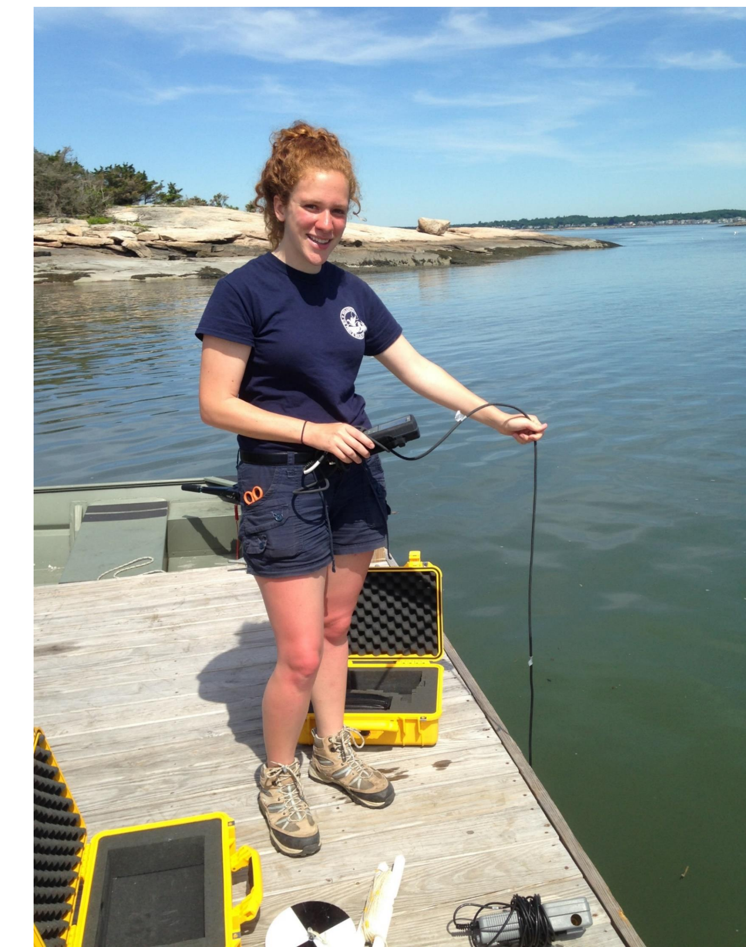
Lauren Gervais deploying a YSI Pro20 to measure dissolved oxygen.
