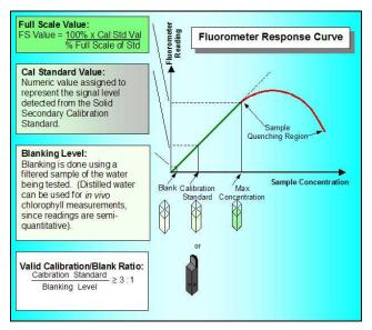
Figure 1. Linearity and Calibration Response Curve
